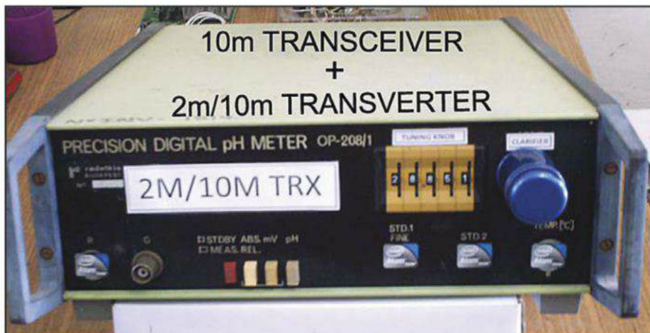
Photo 10. 10-meter transceiver plus 2-meter/10-meter transverter
