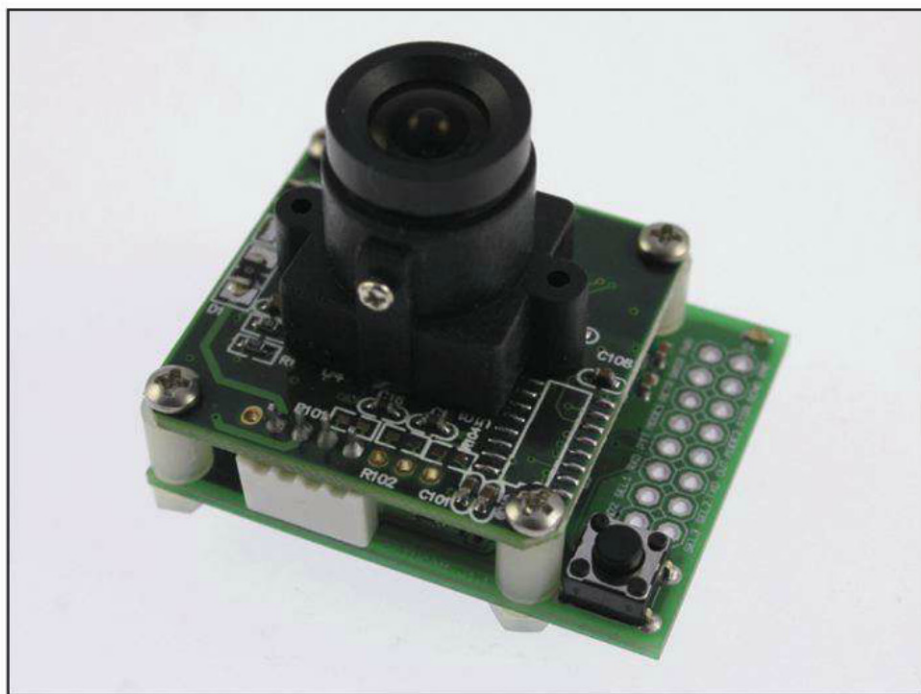
Photo 2. The Argent Data SSTVCAM board. (Photo courtesy of Scott Miller N1VG)
