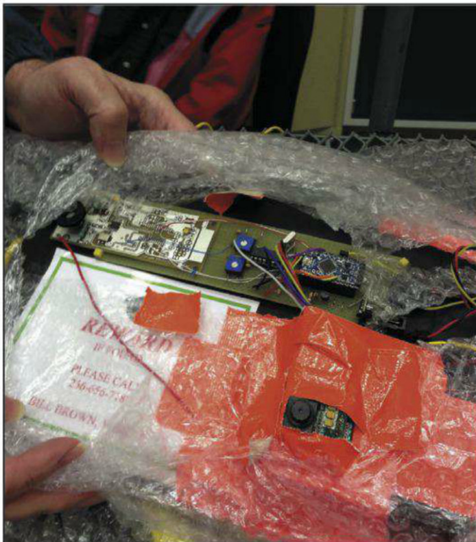
Photo 3. WB8ELK APRS payload with SSTV (real science is not possible without duct tape). (Photo by Bev Teter)
