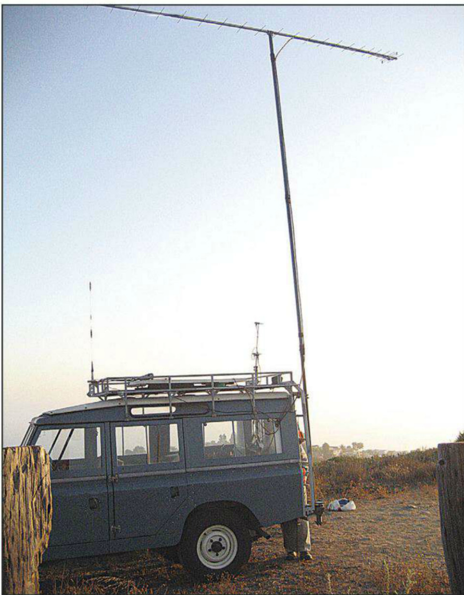
Mobile stations along the West Coast don't need much elevation to access the tropo duct to Hawaii. A clear shot to the west and the ocean is all that is needed!
