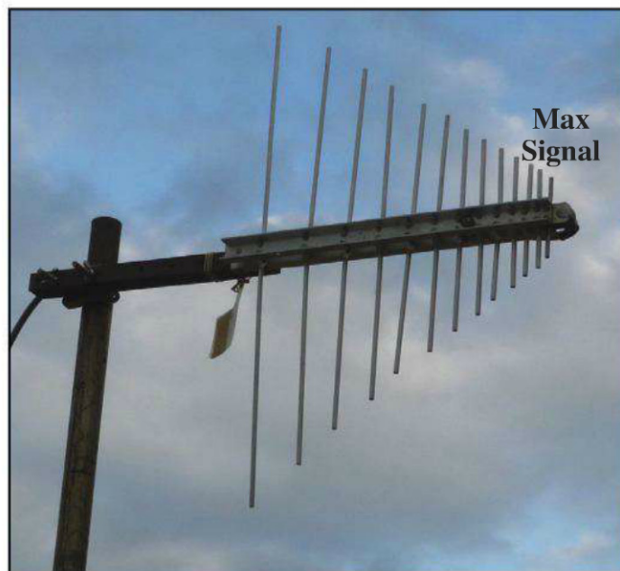
Photo B. Correct way to mount a log periodic
