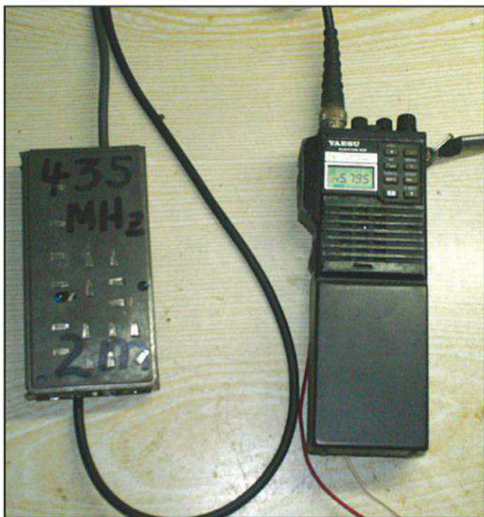
Photo 8. 70-cm down converter plus Yaesu FT-23R HT
