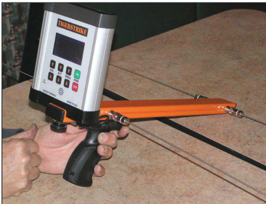
This first-generation TigerStrike RDF set with HB9CV antenna is for tracking ELTs and EPIRBs on the 120-MHz aircraft band. The display shows frequency, bearing, compass heading, and GPS coordinates.
