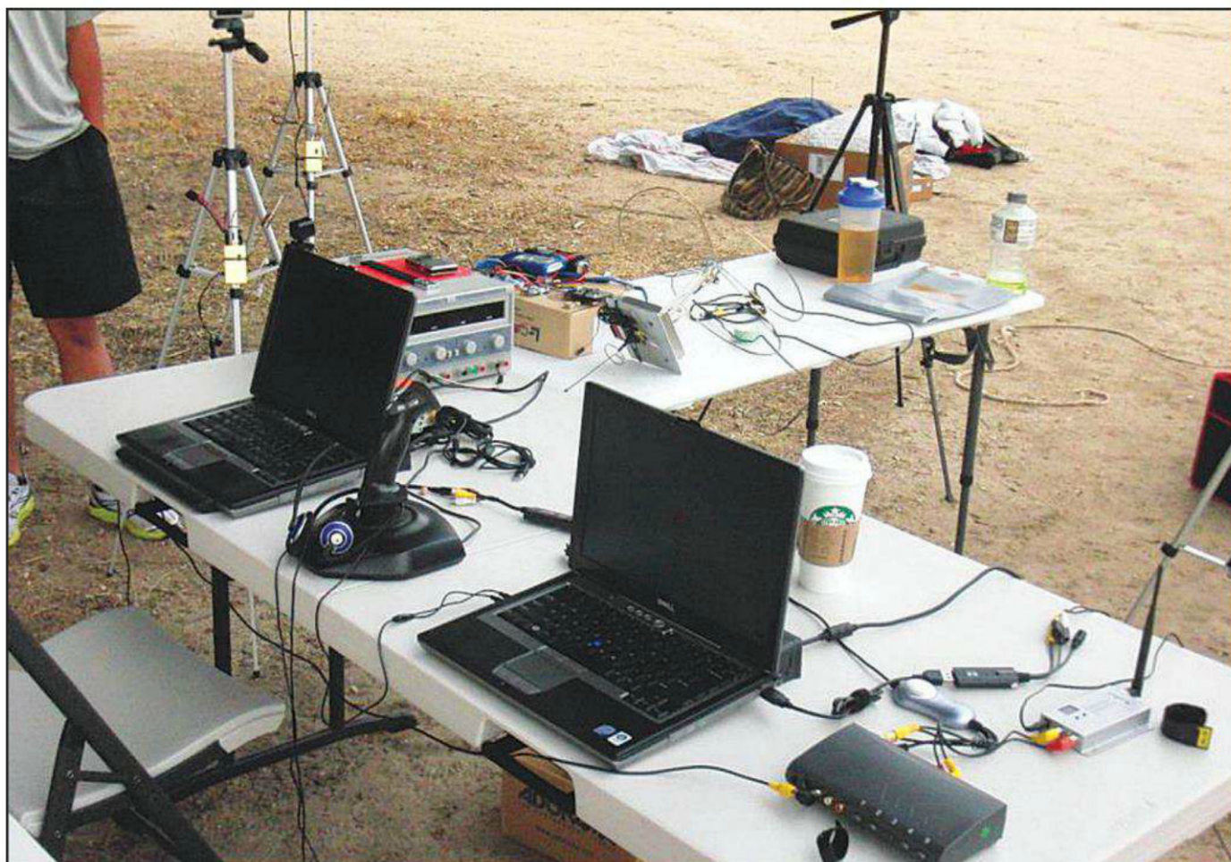
Photo 3. The Quest for Stars internet-connected ground control station system designed for our StratoShuttle UAV flights.
