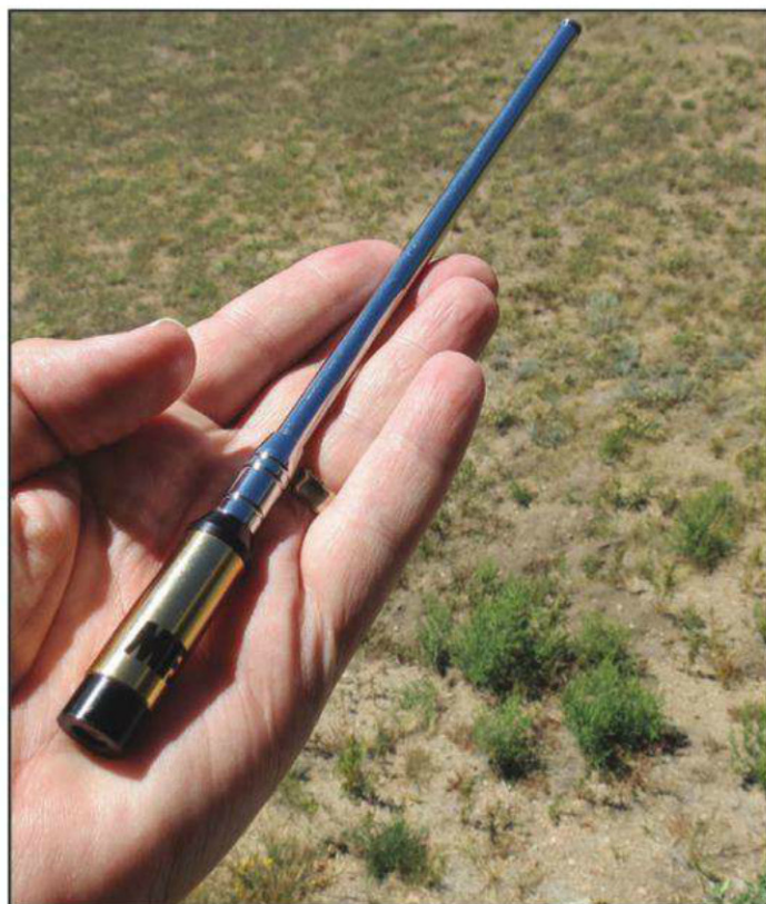
Figure 3. The half-wave antenna collapses down to a convenient size for storage and transportation.
