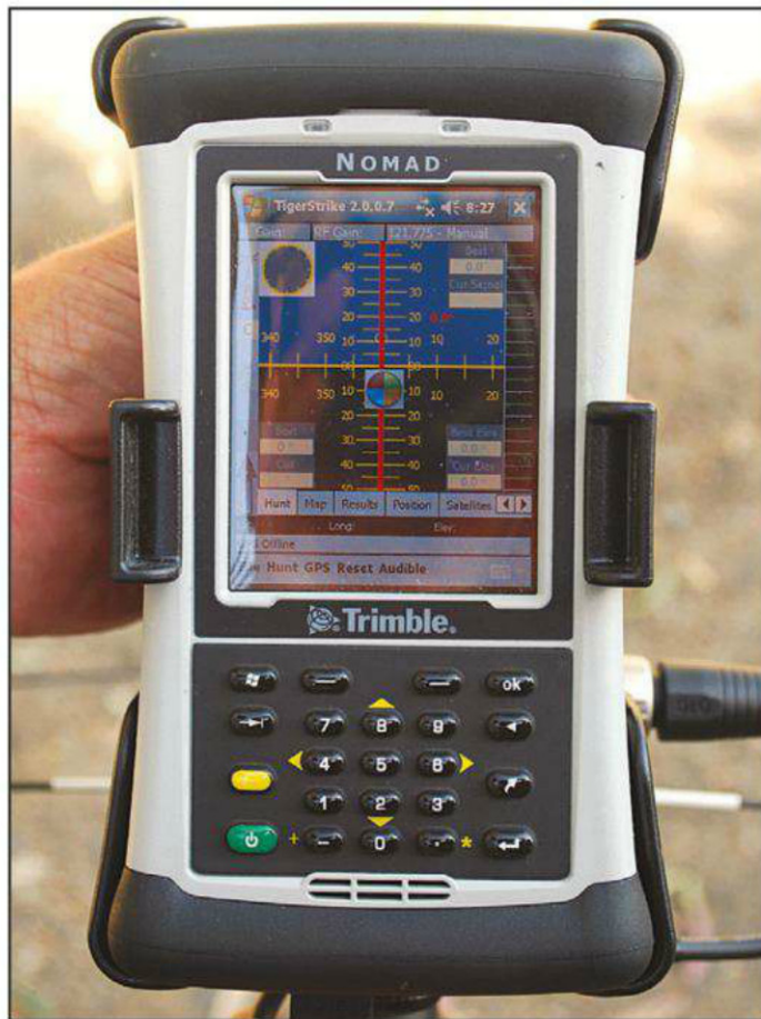
The Trimble Nomad outdoor ruggedized handheld computer as a TigerStrike RDF display unit.
