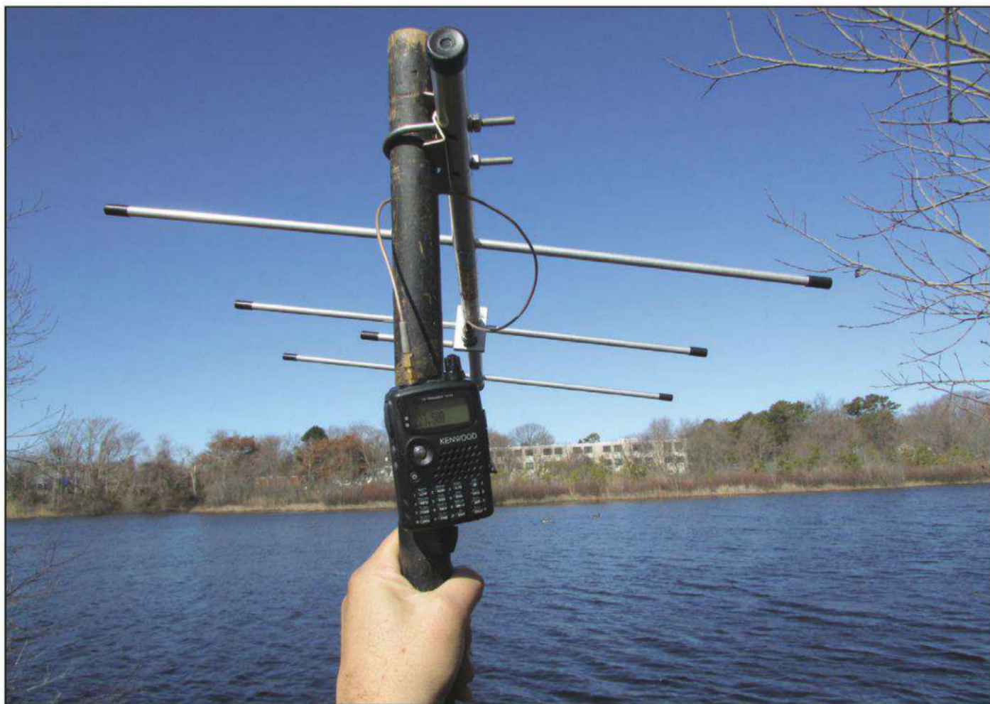
This portable setup for 222 MHz FM consists of a commercially-made 3-element beam that is mounted on a short wooden pole to which the TH-F6 FM HT is mounted. It can quickly be turned by hand toward maximum signal strength.
