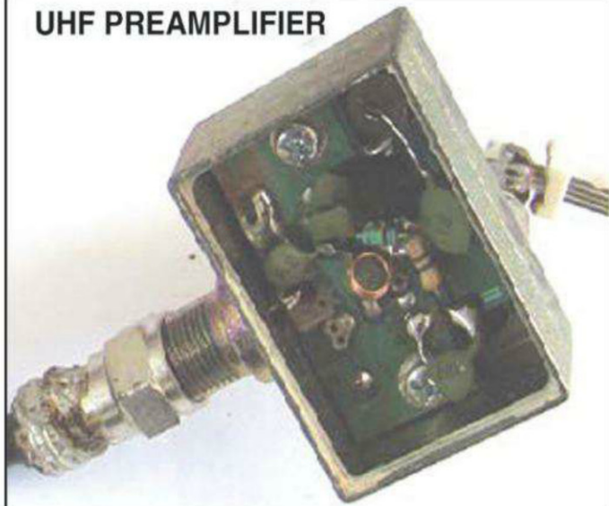
Photo 7A. UHF preamplifier with cover off
