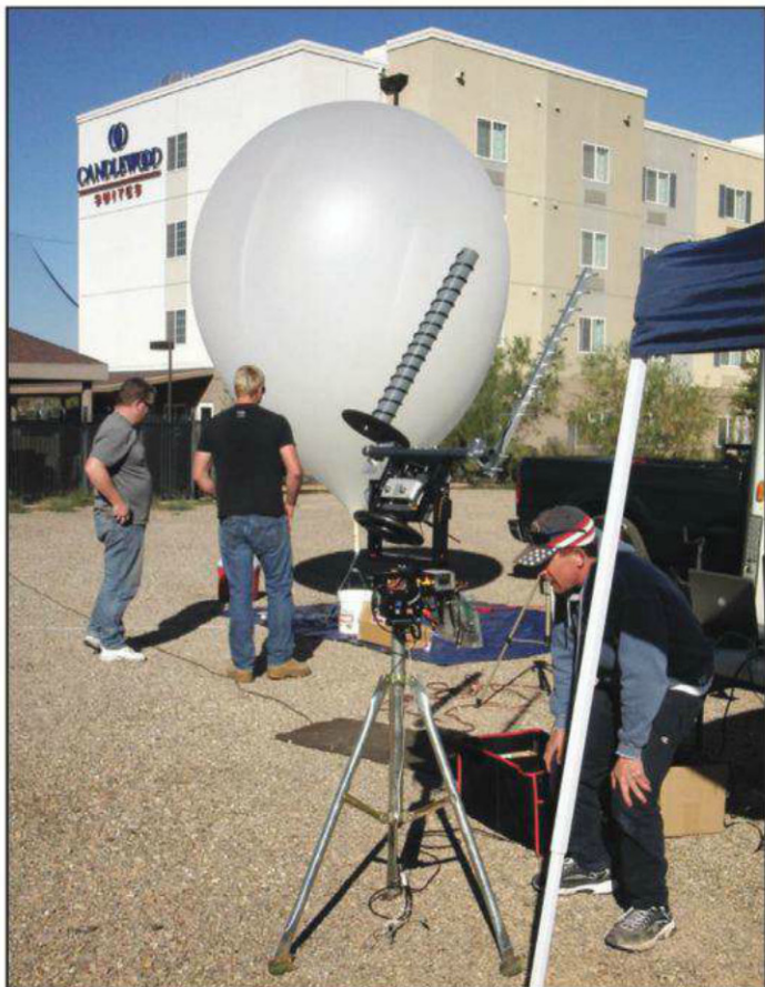
Photo 6. The ground station, rotator, and Stratoshuttle-3 balloon just before launch. Felix was in the air at this point.
