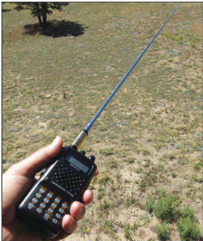
Figure 2. A half-wave antenna for 2 meters is a great improvement over the standard rubber-duck antenna. Shown here is an FT-60 transceiver being used with an MFJ-1714 half-wave antenna.
