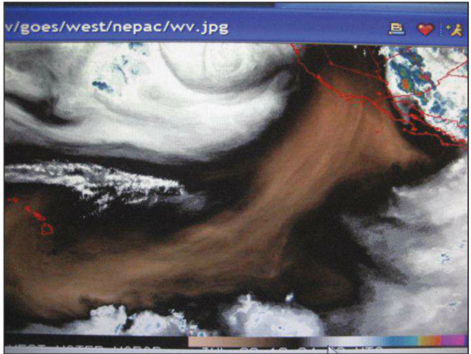
Undisturbed warm air between the mainland US and Hawaii, leading to a strong tropo duct.
